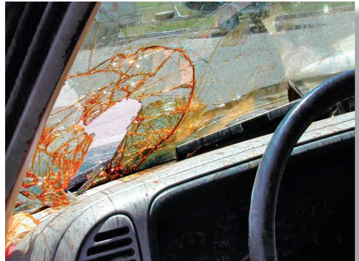
Figure 4. Bear spray canisters can explode as a result of heat buildup if left on the dash of a vehicle, as seen here.
